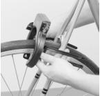
3. Insert strap screws and use to tighten straps around bicycle frame.
